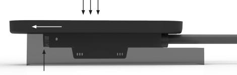
Be sure the fixture is in the forward most position.
